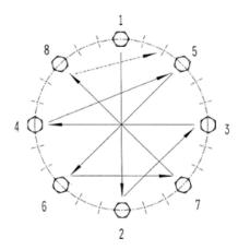
Tighten all fasteners lightly. And tighten to a specified value using a properly calibrated torque wrench; hydraulic devices are advisable.
